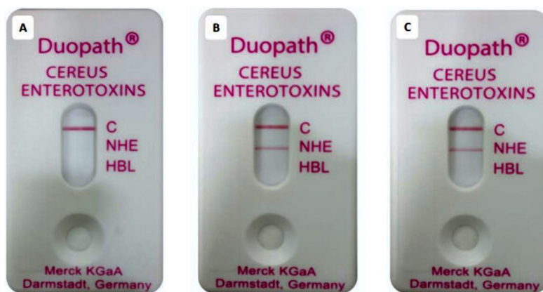
Fig. (5). Image showing Duopath® device after 30 minutes of incubation with respective samples. A: Lactobacillus plantarum 022AE; B: Bacillus cereus ATCC 14579; C: Bacillus cereus ATCC11778.
